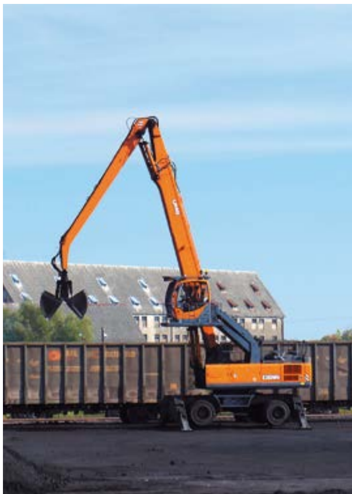
Parametric diagram of E350WH Boom 9,900 mm Main stick 6,900 mm
